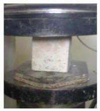
(Fig. 4a) Compressive strength test
