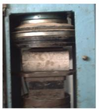
(Fig. 4b) Splitting tensile strength test
