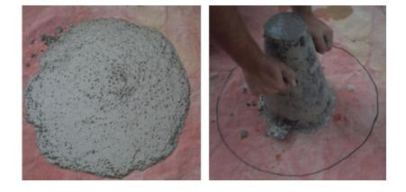
Fig (2) Slump flow test
